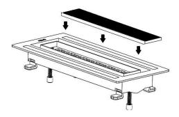
7. Flush the vent cover with the vent flange and place on to the vent hole.
